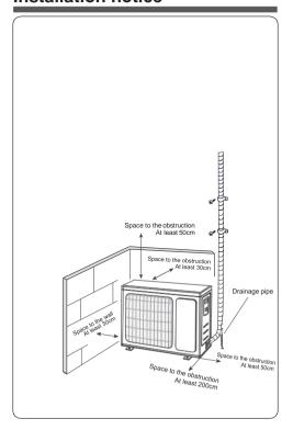
Safety precautions for installing and relocating the unit
